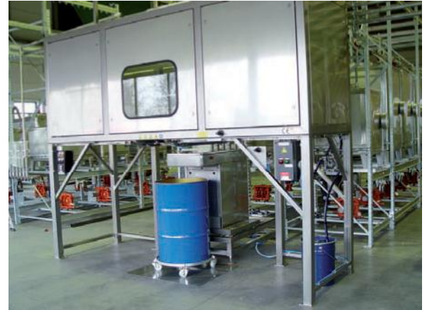
Hybrid Dispensing: gravimetric dispensing system FS 182 with HX5 simultaneous dispenser
