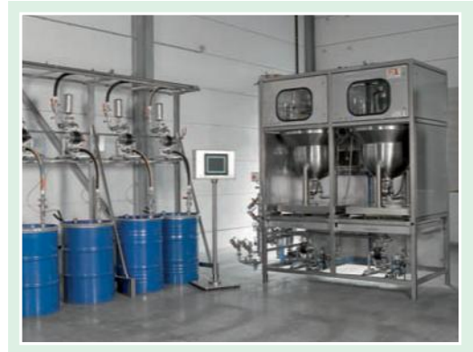
FS 188: semi-continuous supply of reactive silicone components to a dip tank system for the production of silicon implants.
