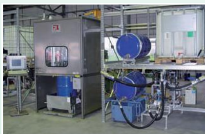
Batch supply of lamination components with integrated agitator for the supply of a lamination machine.
