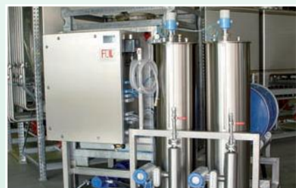
Continuous supply of lamination components via mass flow meter to a curtain coater for the production of packaging material for the food industry.
